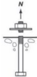
(i) Steel failure
